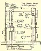
Fig. 232.—Mechanical remotecontrol circuit-breaker mounted on wall.
